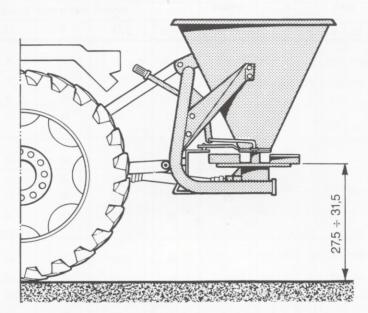
Before operating the spreader, make sure that the spreading disc is set to the horizontal position and at about  $27.5 \div 31.5$  in from ground level.
